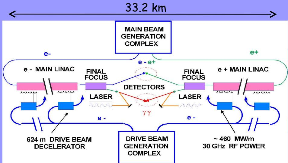
■ High acceleration gradient (150 MV/m)
