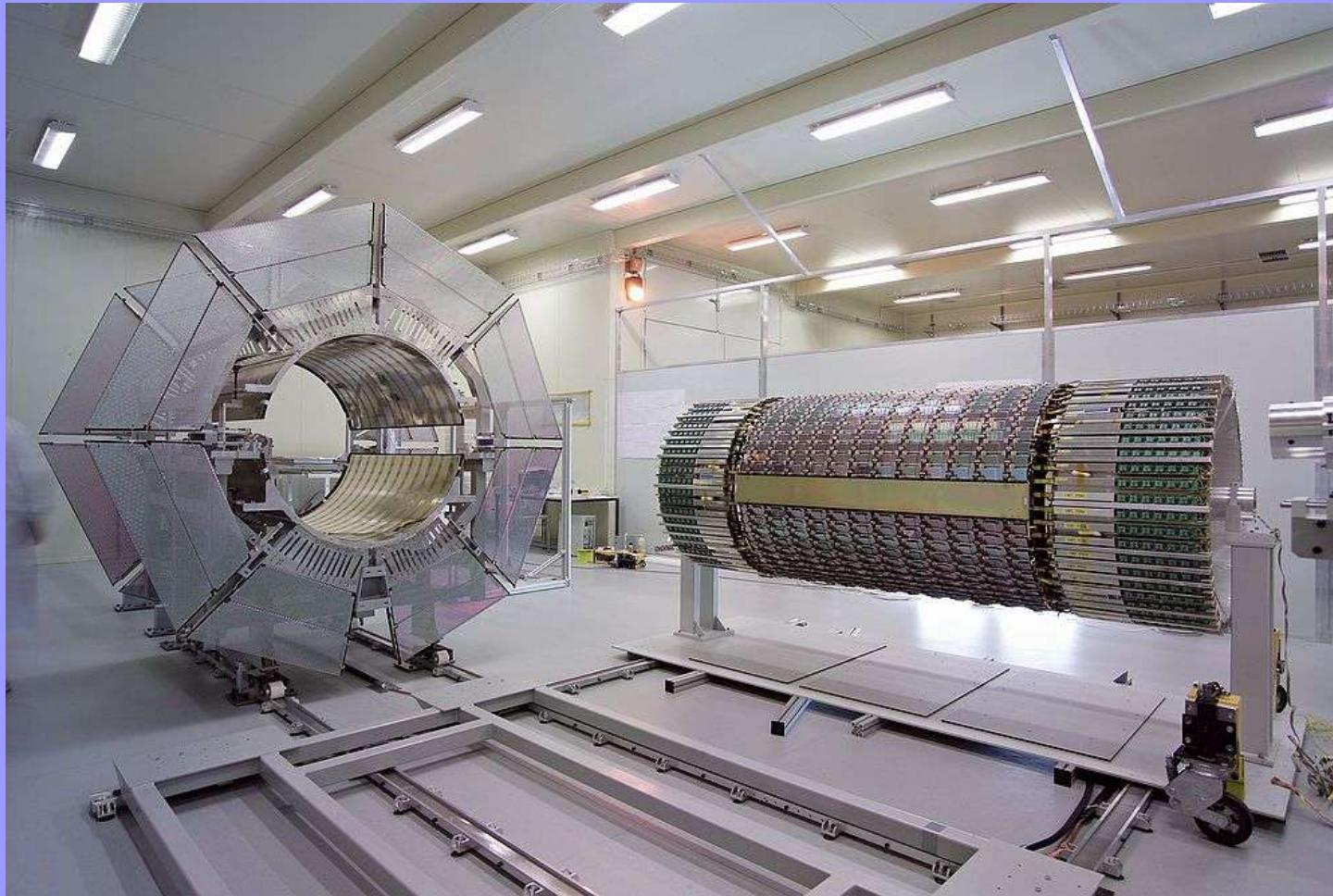
Outermost ATLAS SCT barrel cylinder before insertion into the support structure
